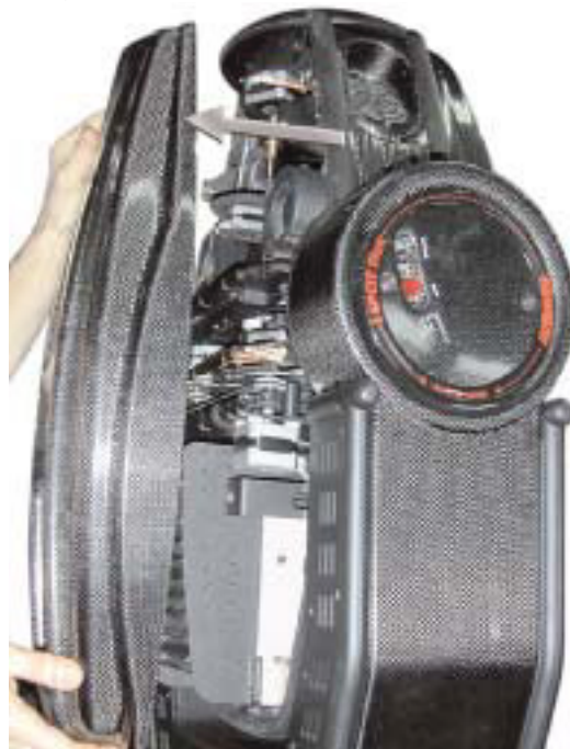
Figure W12B Removing Fixture Covers
