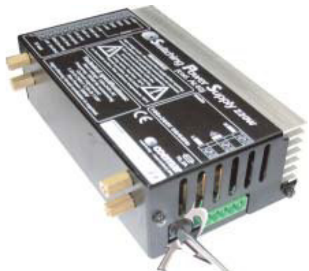
Figure W11D - Changing Switching Supply Fuse
